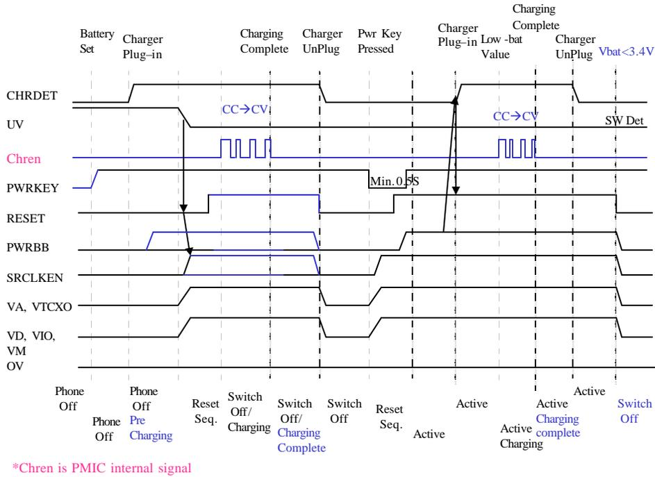
Figure 5 Charger State Timing
