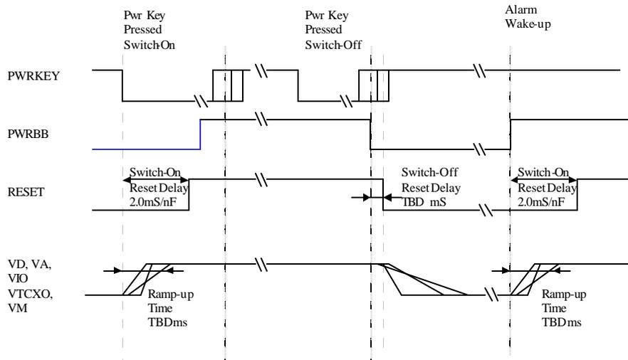
Figure 6 Reset Timing
