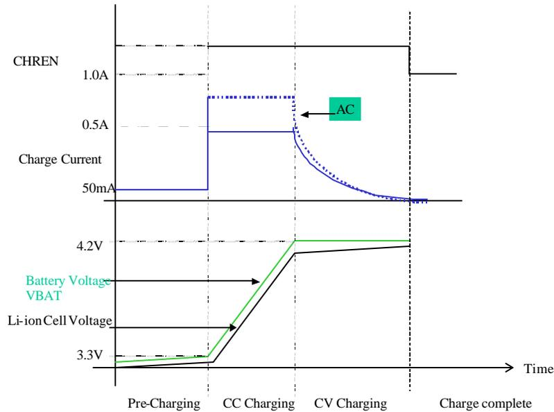
Figure 9 I-V curve of Li-Ion Battery Charging
