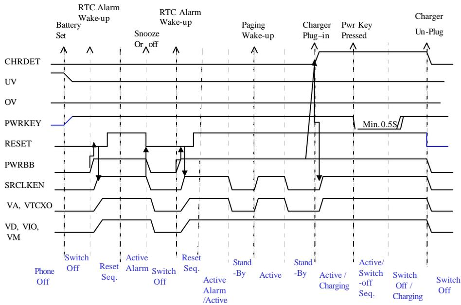
Figure 4 State Timing for Wake up, Paging and Stand-by
