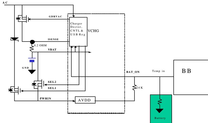
Figure 15 BAT\_ON connection with Battery Temp. sensor example
