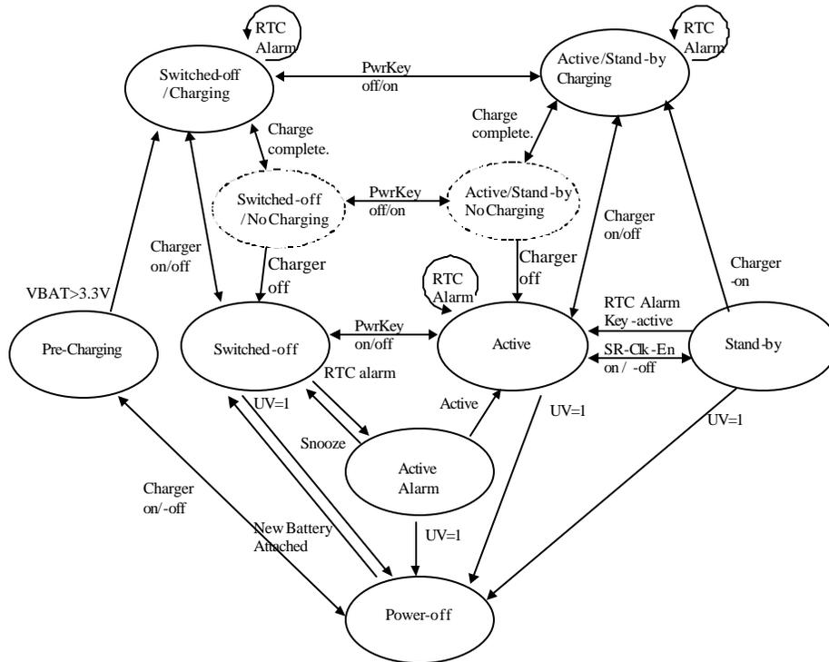
Figure 1 Power Management State Diagram
