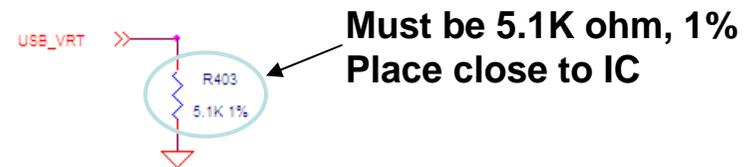
For USB/ standard charger detection, **Different from MT6238**
